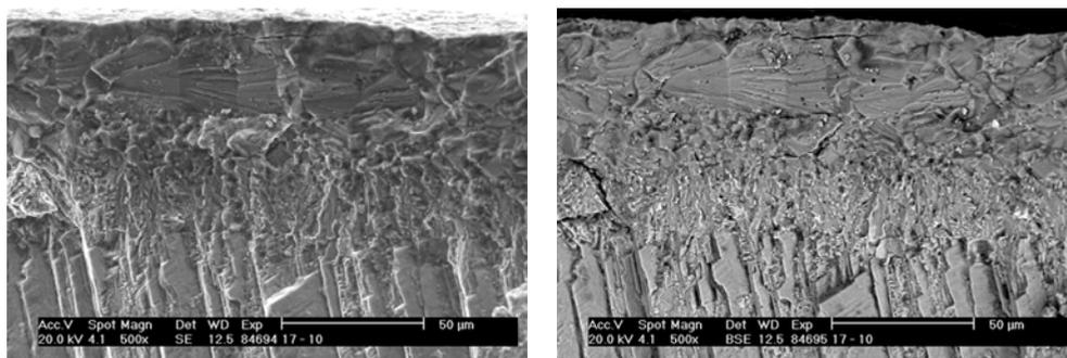
Fig.2. Detail of an initiation site within aluminide diffusion coating in Inconel 713LC specimen subjected to combined bending-torsion loading ( $\sigma_a = 289$  MPa,  $\tau_a = 233$  MPa,  $N_f = 6.0 \times 10^4$  cycles).
