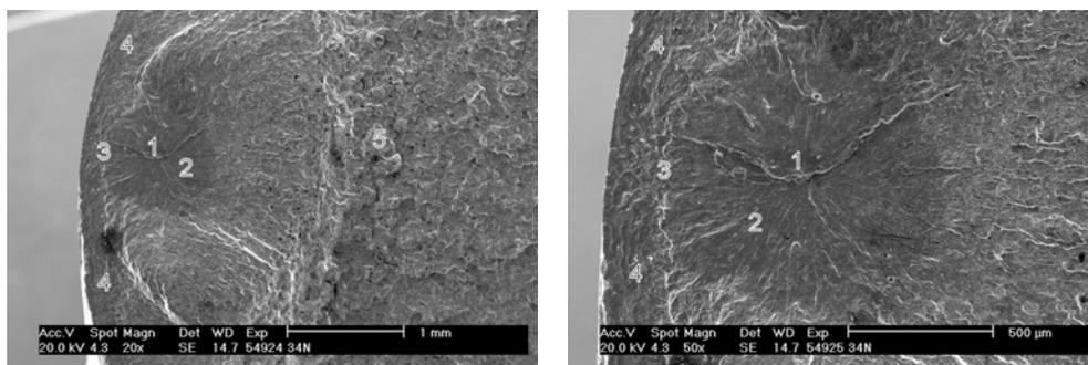
Fig.1. Fish-eye type failure in nitrided steel specimen subjected to combined bending-torsion loading ( $\sigma_a = 510 \text{ MPa}$ ,  $\tau_a = 510 \text{ MPa}$ ,  $N_f = 2.0 \times 10^5$  cycles).
