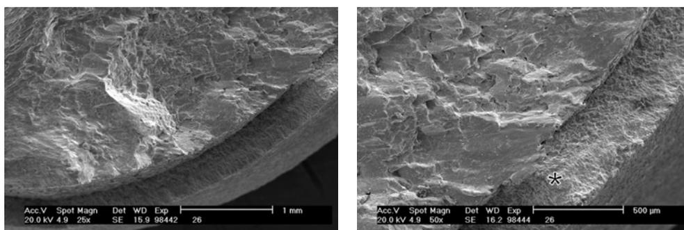
Fig.3. Detail of an initiation site (indicated by a star) within thermal barrier coating in Inconel 713LC specimen subjected to combined bending-torsion loading ( $\sigma_a = 264$  MPa,  $\tau_a = 272$  MPa,  $N_f = 4.2 \times 10^4$  cycles).
