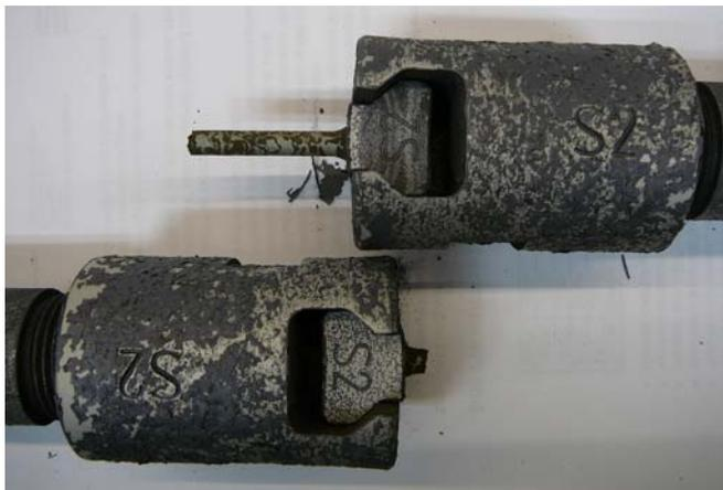
Fig.1. Image of damaged creep machine grips after the test.
