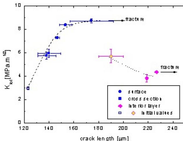
Fig.5. Total stress intensity factor ( $K_{tot}$ ) vs crack length in four-point bending load tests.
