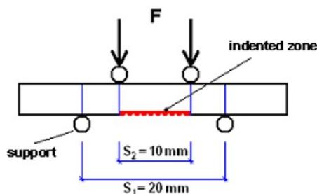
Fig.3. Schematic of 4-point bending test.
