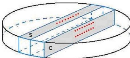
Fig.2. Schematic view of indented bars S (surface) and C (cross section).
