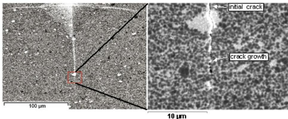
Fig.6. Micromechanisms of crack growth. Character of the initial indentation crack and the slow crack growth path, although the latter is more intergranular, is very similar. Even occasional clusters of zirconia grains (light coloured) do not change it significantly.
