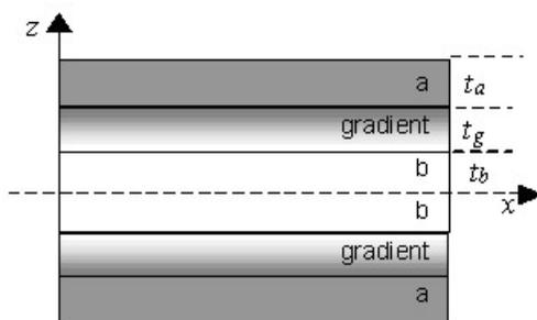
Fig.1. Schematic of symmetrical planar functionally graded material with layer thickness  $t_a$ ,  $t_b$ , and  $t_g$ , respectively.
