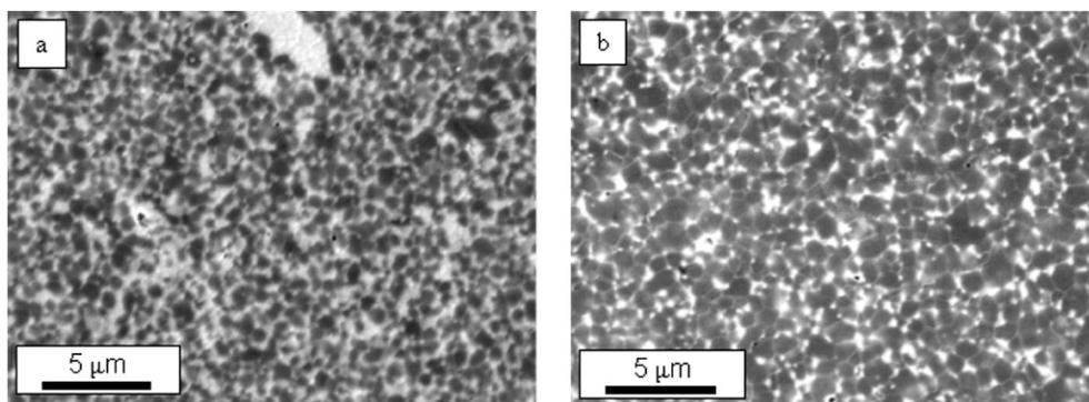
Fig.4. Microstructure of the homogeneous layers of the experimental material. (a) Central layer; (b) outer layer.
