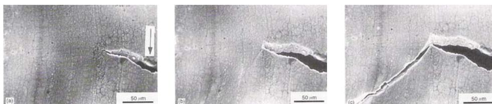
Fig.3. Propagation of the fracture toward the specimen interior: a) elongation 0.12 mm; b) elongation 0.18 mm; c) elongation 0.185 mm.
