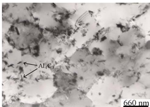
Fig.1.  $\text{Al}_4\text{C}_3$  particles identified by TEM.
