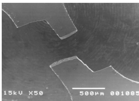
Fig.6. Final fracture by interconnecting the two opposite side cracks in the material with 12 vol.%  $\text{Al}_4\text{C}_3$  ( $\epsilon=0.05$ ).
