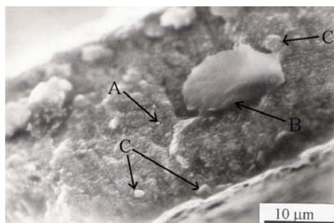
Fig.7. Surface morphology of the material with 12 vol.%  $\text{Al}_4\text{C}_3$  ( $\epsilon=0.05$ ).
