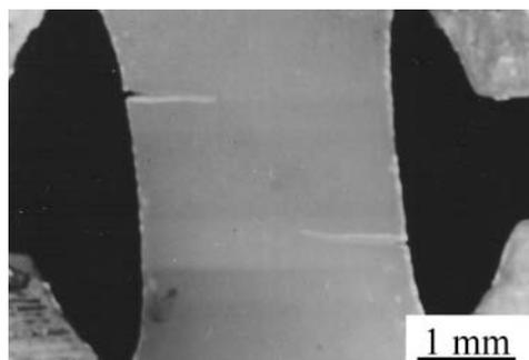
Fig.5. Two cracks initiated on the opposite sides of a specimen. Surface morphology and initiation of cavities in the matrix-particle interphase in the material with 12 vol.%  $\text{Al}_4\text{C}_3$  ( $\epsilon=0.04$ ).
