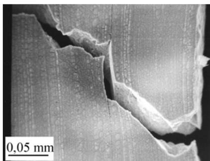
Fig.4. Irregular fracture formed by a crack growing alternately along the particle rows and between them in the material with 8 vol.%  $\text{Al}_4\text{C}_3$  ( $\epsilon=0.15$ ).
