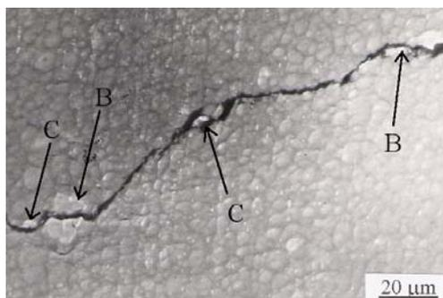
Fig.2. Fracture path in the material with 8 vol.%  $\text{Al}_4\text{C}_3$ . Rupture of a large  $\text{Al}_4\text{C}_3$  grain and decohesion of the smaller particles ( $\epsilon=0.12$ ).
