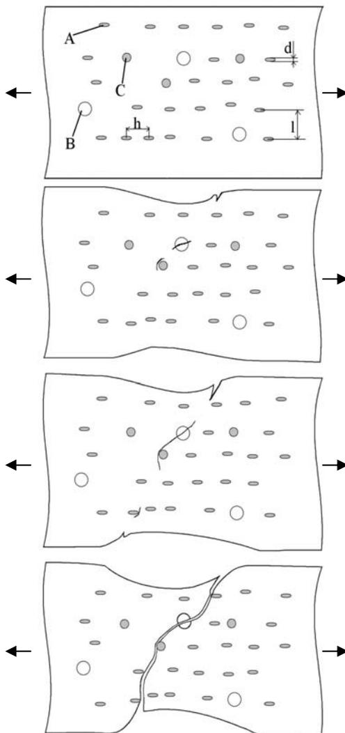
Fig.8. Model of the fracture mechanism.
