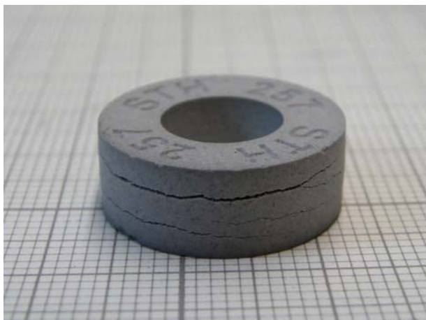
Fig.7. Cracked PTCR after sintering with high heating rate in laboratory furnace.
