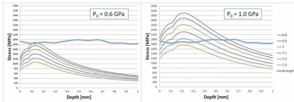
Fig.3. Theoretical prediction of the effect of density on the contact fatigue resistance of the sinterhardened Fe-1Mo-2Cu-0.65C steel at 0.6 GPa and 1.0 GPa mean pressure.
