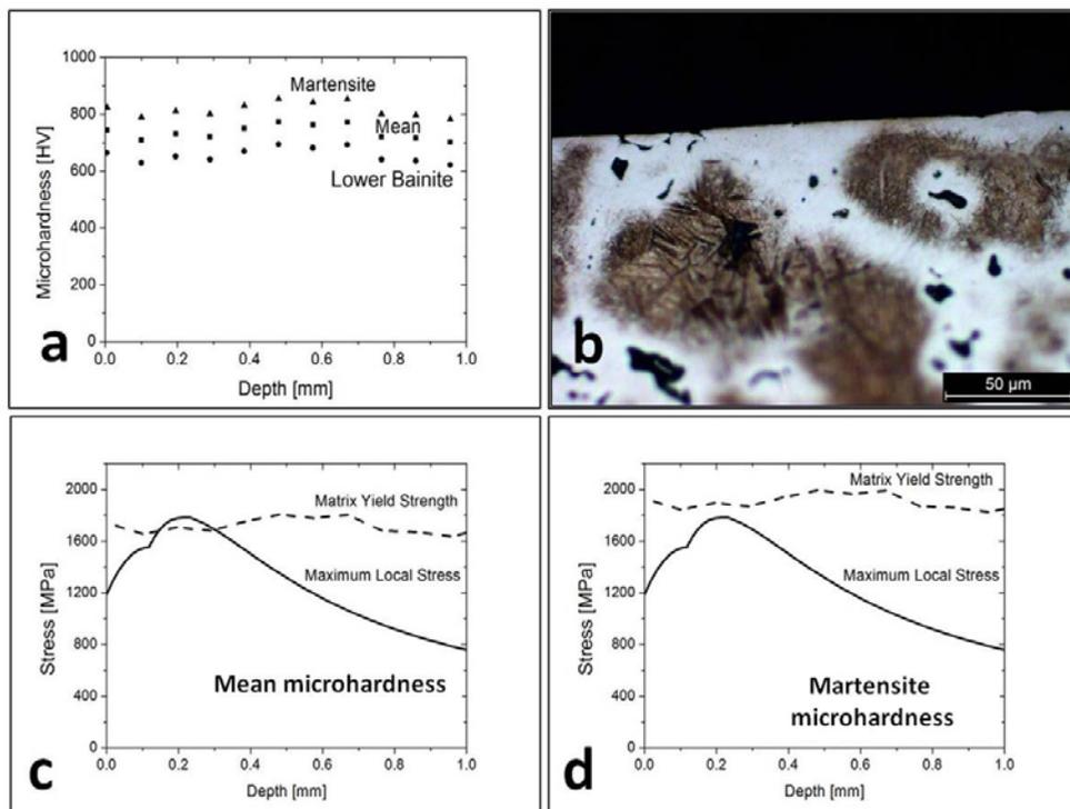
Fig.2. Microhardness profile (a), microstructure of the tested specimen (b), profile of maximum local stress and of matrix yield strength calculated from the mean microhardness (c) and from the microhardness of martensite (d) for sinterhardened Fe-1Mo-2Cu-0.65C steel at  $P_0 = 1$  GPa.
