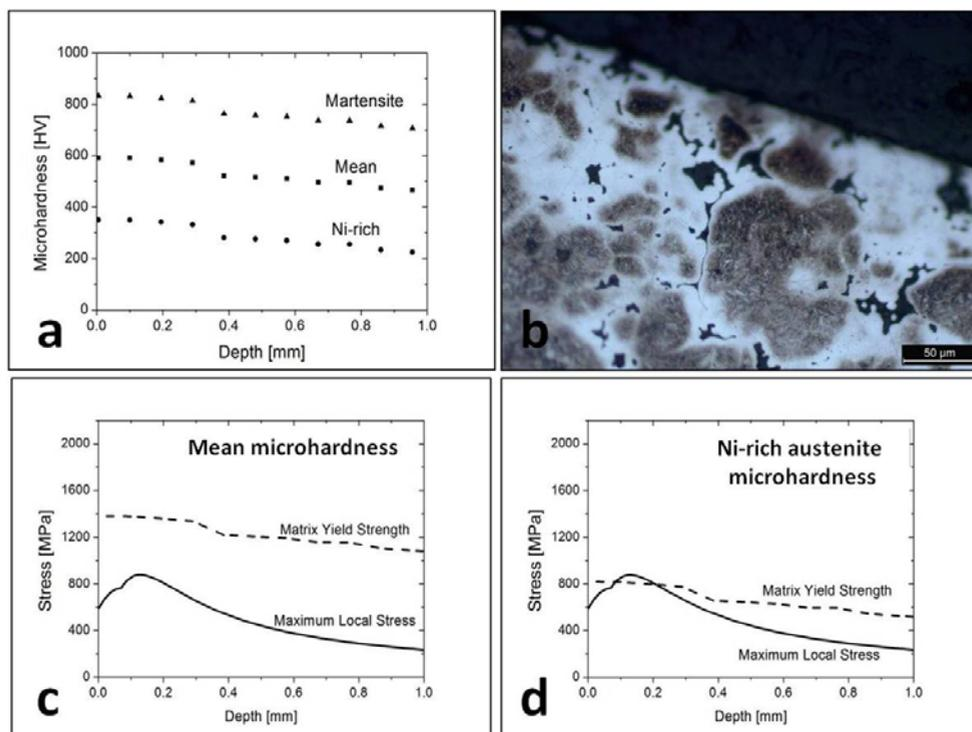
Fig.1. Microhardness profile (a), microstructure of the tested specimen (b), profile of maximum local stress and of matrix yield strength calculated from the mean microhardness (c) and from the microhardness of Ni-austenite (d) for heat treated Fe-4Ni-0.5Mo-1.5Cu-0.5C steel at  $P_0 = 0.6 \text{ GPa}$ .
