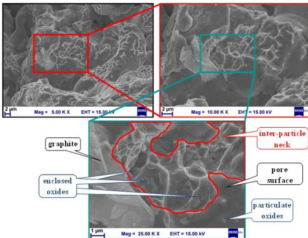
Fig.3. Inter-particle neck region,  $AstCrM+0.4\%C$  compact heated in  $N_2/10\%H_2$  to  $900^\circ C$ , showing enclosure of surface oxide residue inside growing inter-particle neck.
