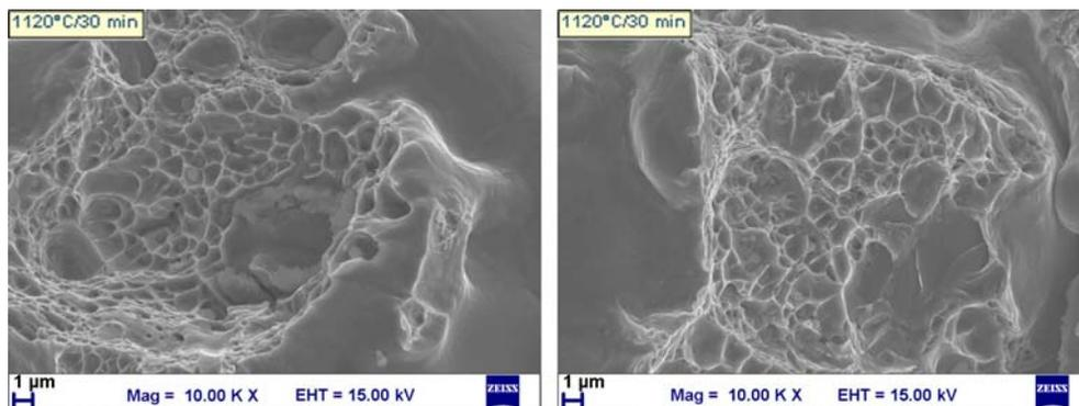
Fig.1. Fracture surface of AstCrA+0.5%C compacts sintered at to 1120°C for 30 min in nitrogen (left) and nitrogen/hydrogen (right) atmospheres.
