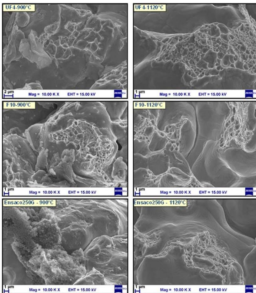
Fig.4. Fracture surface of  $AstCrM+0.5\%C$  compacts utilizing different carbon sources, heated in  $Ar/10\%H_2$  to 900 (left) and 1120°C (right), showing development of inter-particle necks.
