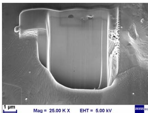
Fig.2. Surface oxide on water-atomized low alloy steel powder (Fe-3Cr-0.5Mo) revealed by means of FIB-SEM [27].
