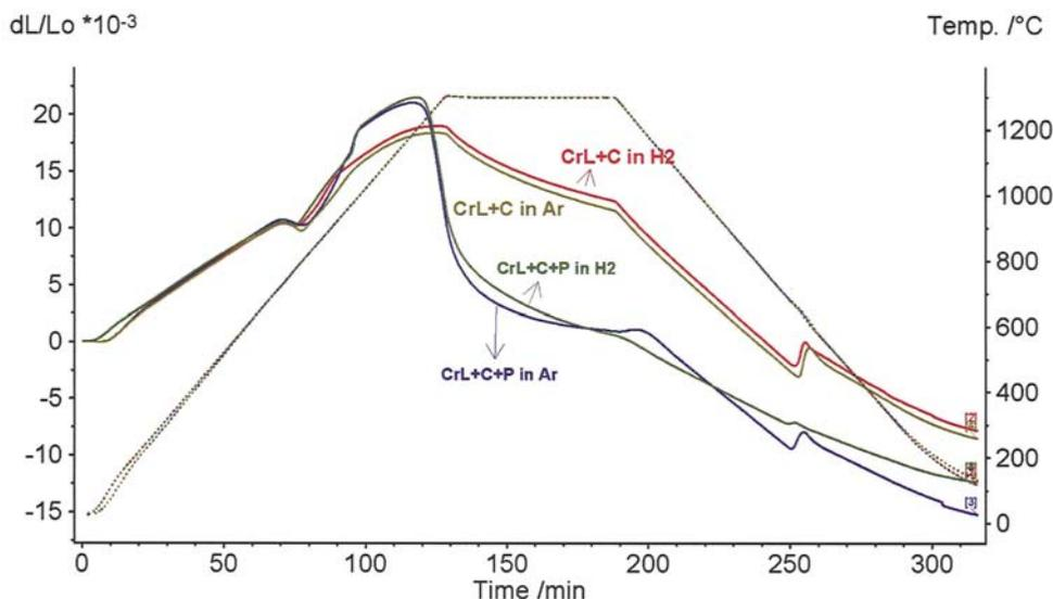
Fig.1. Dilatometric graphs of AstaloyCrL-0.6%C(-0.45%P) sintered in  $H_2/Ar$  respectively. 10 K/min / 60 min 1300°C / -10 K/min.
