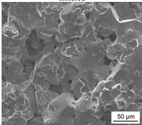
Fig.8e. AstaloyCrL-0.6%C-0.45%P, sinter hardened
