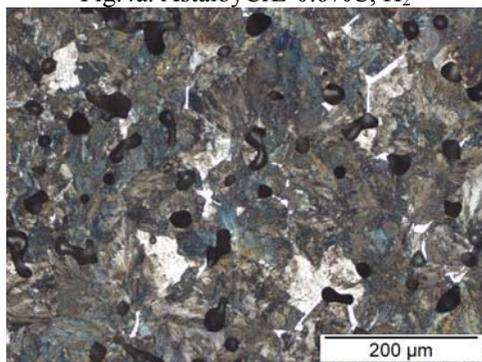
Fig.4c. AstaloyCrL-0.6%C-0.45%P, H<sub>2</sub>
