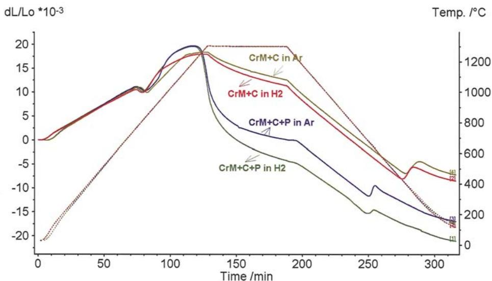
Fig.2. Dilatometric graphs of AstaloyCrM-0.6%C(-0.45%P) sintered in H<sub>2</sub>/Ar respectively. 10 K/min / 60 min 1300°C / -10 K/min.
