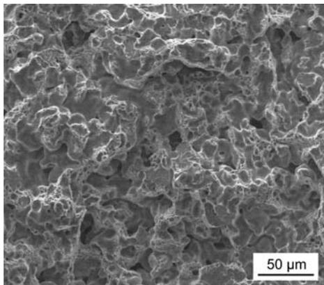
Fig.8a. AstaloyCrL-0.6%C, as sintered
