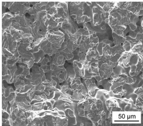
Fig.8b. AstaloyCrL-0.6%C-0.45%P, as sintered
