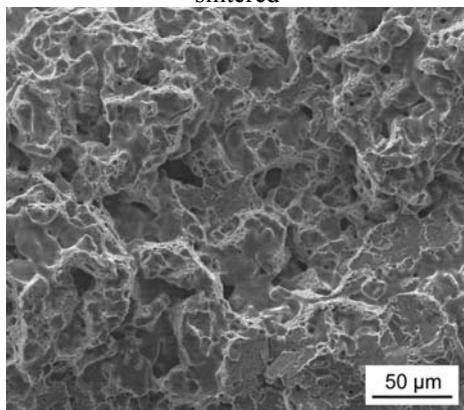
Fig.8d. AstaloyCrL-0.6%C, sinter hardened
