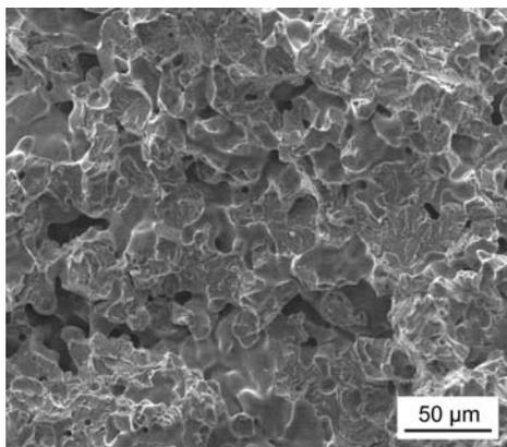
Fig.8c. AstaloyCrM-0.5%C-0.45%P, as sintered
