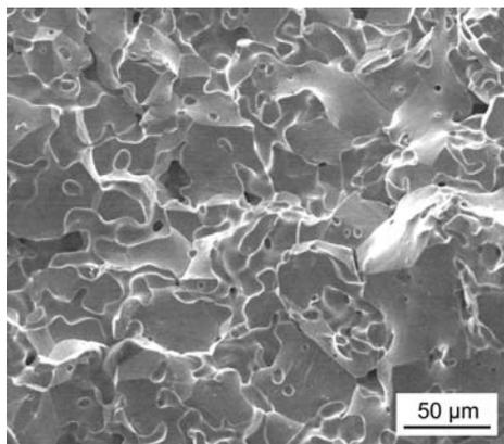
Fig.8f. AstaloyCrM-0.5%C-0.45%P, sinter hardened
