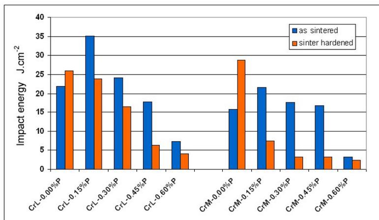
Fig.7. Charpy impact energy of AstaloyCrL/CrM-C(-P) specimens sintered/sinter hardened in the push-type furnace. Compacted at 600 MPa, sintered 60 min at 1250°C in H<sub>2</sub>, sinter hardened at 2 K·s<sup>-1</sup> in N<sub>2</sub>.
