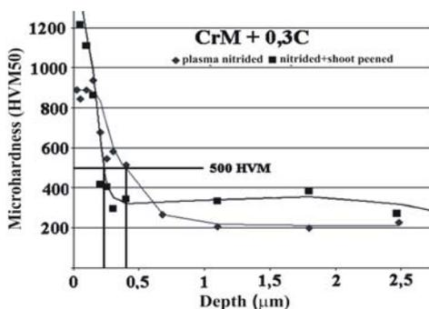
Fig.8. Behaviour of the cross-sectional microhardness of Ast CrM + 0.3% C material.
