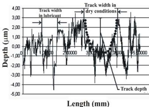
Fig.12. Example of the profilograph running along the track following the wear of Ast CrM + 0.3% C material with lubricant and without lubricant.
