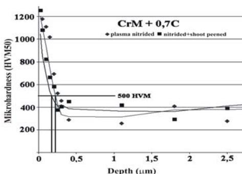
Fig.9. Behaviour of the cross-sectional microhardness of Ast CrM + 0.7% C material.
