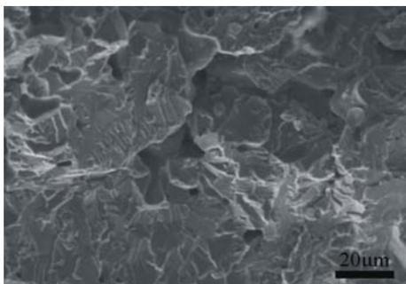
Fig.6. The area below the surface and fracture cleavage facets of brittle fracture.
