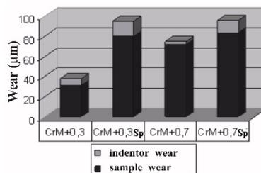
Fig.16. Indenter and material wear test in lubricant.
