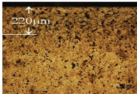
Fig.5. Microstructure of Ast CrM + 0.7% C.
