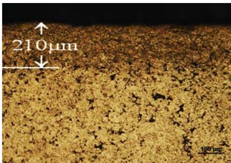
Fig.2. Microstructure of Ast CrM + 0.3% C. Shot peened + nitrided.
