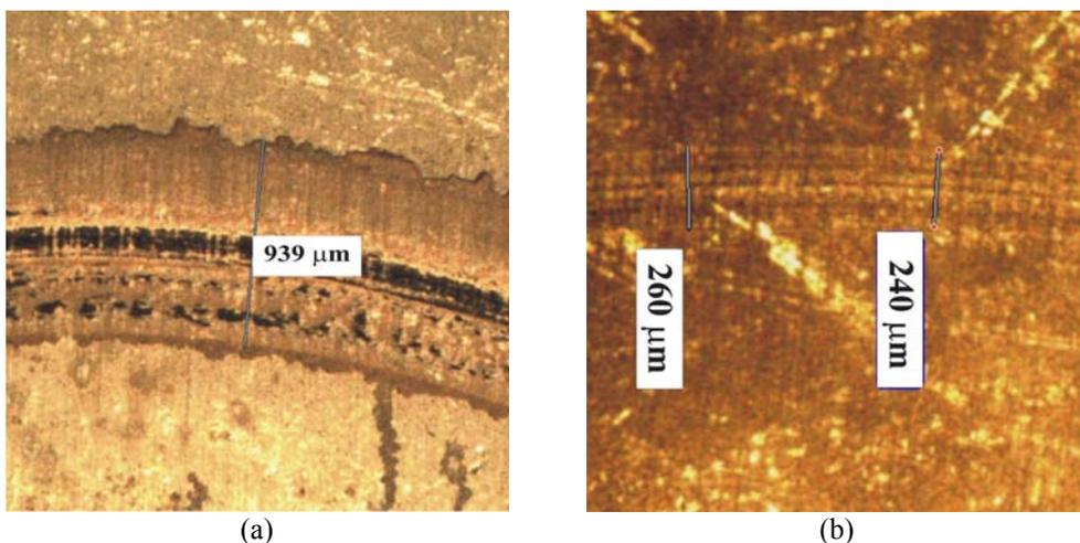
Fig.14. The appearance of wear after riding on a sample of 360 m without and with lubricant - material Ast CrM + 0.7% C.
