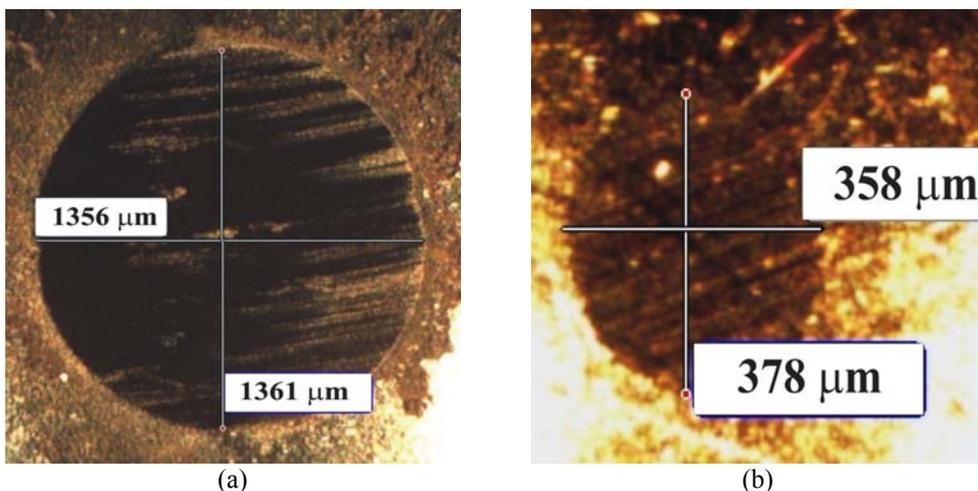
Fig.13. The appearance of the indenter wear after riding 360 m without and with lubricant - material Ast CrM + 0.3% C.
