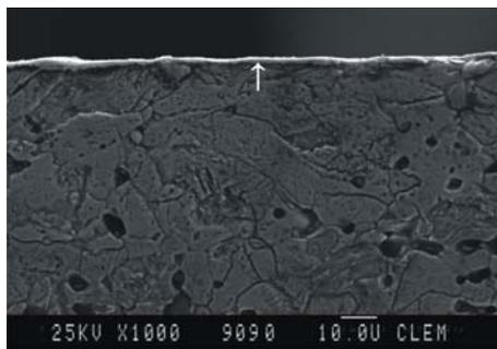
Fig.7.  $\epsilon$  - layer on the surface of plasma nitrided material.
