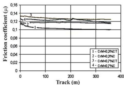
Fig.11. Friction coefficient – in lubricant.
