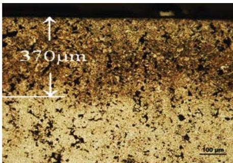
Fig.4. Microstructure of Ast CrM + 0.3% C.
