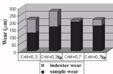
Fig.15. Wear materials and indenter test in dry conditions.
