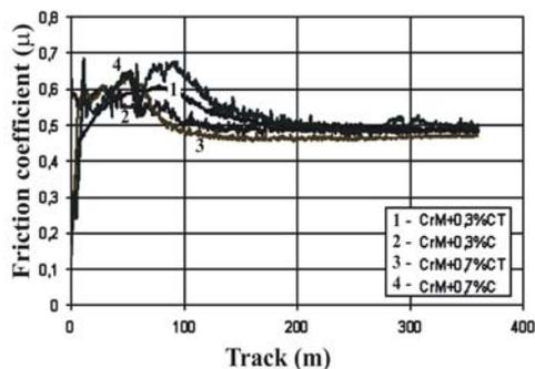
Fig.10. Friction coefficient - dry conditions.
