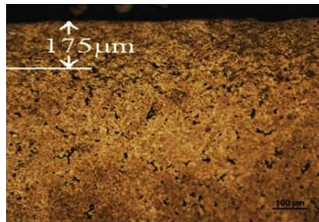
Fig.3. Microstructure of Ast CrM + 0.7% C – Sp. Shot peened + nitrided.
